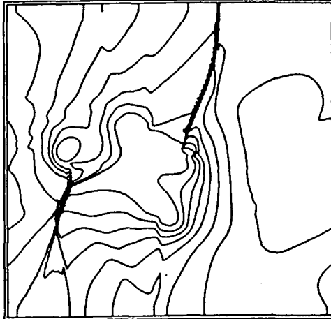
Figure 33: Contour lines of the four-vortex simulation, Ma_c = 0.8 , Re = 1000 , Pr = 0.7 , L_x = 80 \cdot \delta_i , t = 400
