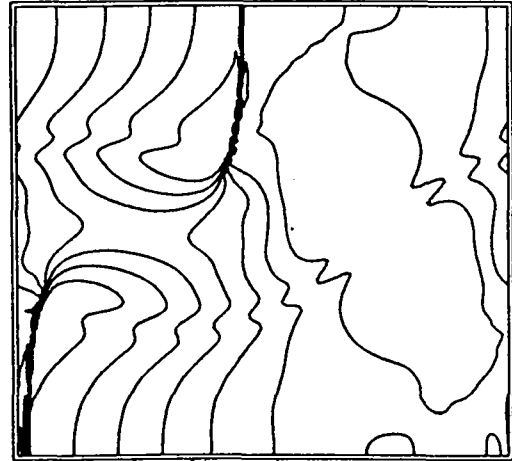
Figure 9: Contour-lines with 201 points in x-direction, Ma_c = 0.8 , Re = 400 , Pr = 0.7 , L_x = 20 \cdot \delta_i , t = 80
