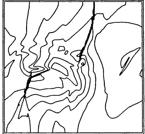
Figure 33: Contour lines of the four-vortex simulation, Ma_c = 0.8 , Re = 1000 , Pr = 0.7 , L_x = 80 \cdot \delta_i , t = 400
