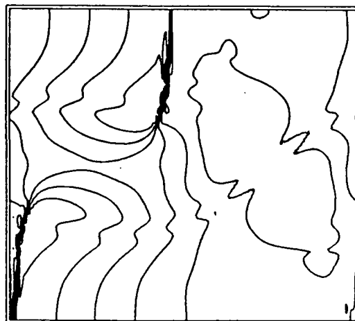
Figure 8: Contour-lines with 101 points in x-direction, Ma_c = 0.8 , Re = 400 , Pr = 0.7 , L_x = 20 \cdot \delta_i , t = 80
