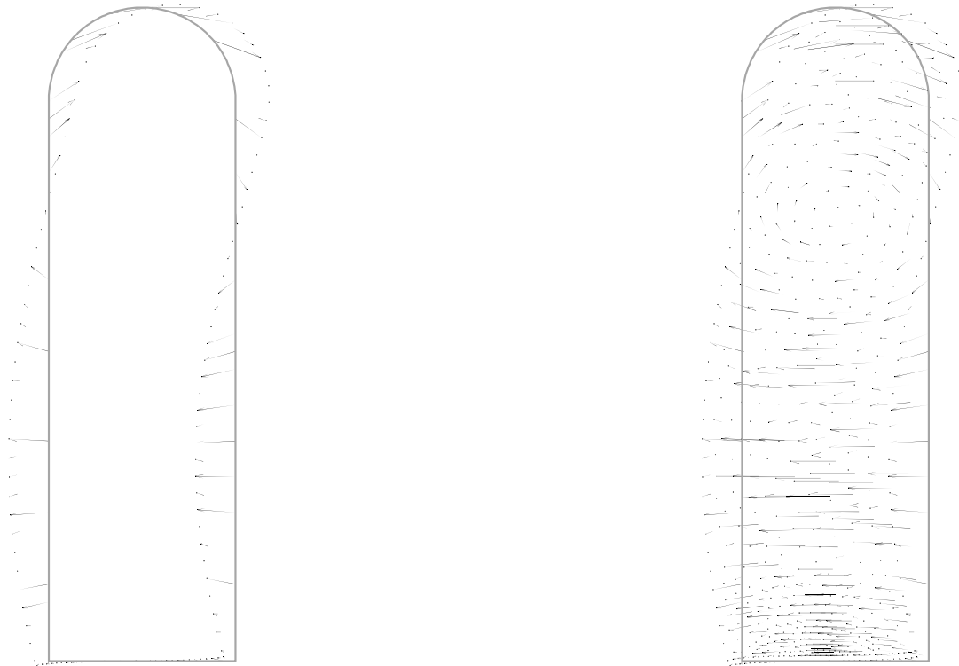
FIG. 9.36 - COMPOSANTES TRANSVERSALES DU 2 ème MODE / \beta = 10 / \omega = 2.603 / \tau = 0.25
