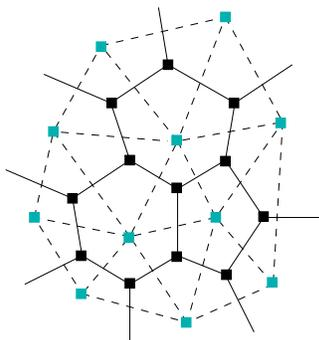
Figure 2: Surface simplex mesh duality with triangulations.
