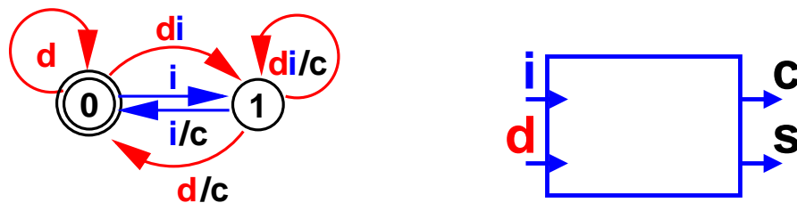
Figure 1: The behaviours of a 1-bit counter, and its input-output profile.
