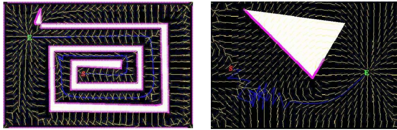
Figure 8: Showing how the method may be adapted to different strategies. In the left view, we have considered a case where the potential function already represents the full geometry of the environment: in that case the algorithm does not modify the potential, while we obtain a smoother trajectory in the “median way”. In the right view, we have considered adding spread of boundary locations within the “line of sight” (see text for details): the method still works in this case.
