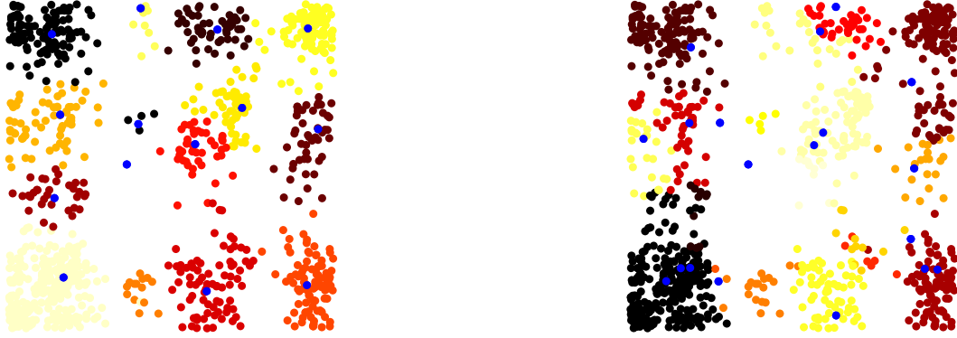
Figure 12: Non uniform distribution of nodes: Example of clusters organization for 1000 nodes with a radius R = 0.1km with the 1-density heuristic (a) and with the Max Min 3-cluster (b).
