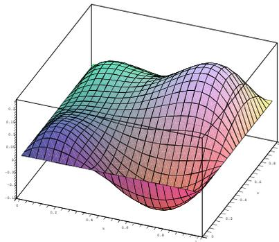
Figure 14: Plot of the degree 4 Bezier surface
