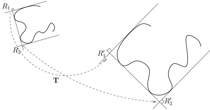
Figure 14: Two pieces of level lines and their corresponding local similarity frames. The similarity  $\mathbf{T}$  maps  $R_1$  into  $R'_1$  and  $R_2$  into  $R'_2$ . Equivalently the local frame,  $(R_1, R_2)$  may be represented by  $(p, v) = (\frac{R_1+R_2}{2}, R_2 - R_1)$ .
