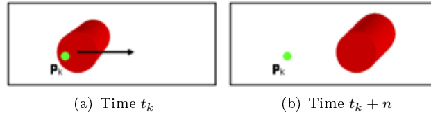
Figure 6: Record k is created at time t_k on the dynamic object. Even though the object moves in subsequent frames, record k remains at the same position.
