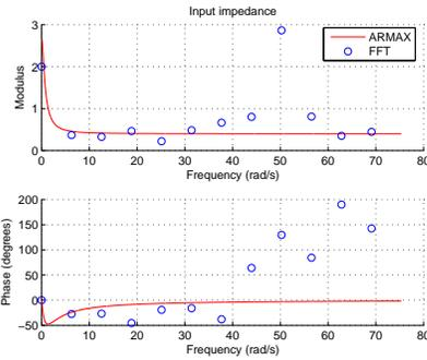
Fig. 9. Input impedance at human aorta : ARMAX and FFT approaches.
