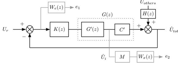
Fig. 5.  $H_\infty$  design bloc diagram
