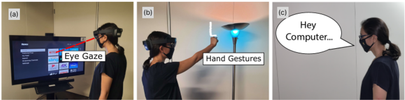
Figure 3: Different modalities of interaction with affordances [14]. In (a), the affordance is represented by a highlight on the screen on the elements selected by the visual interaction, guiding the user as to which elements are interactive. In (b), the affordance is displayed on the HMD anchored in the environment, showing a graphic element that indicates the gesture necessary for the interaction to occur. In (c), sound affordances are activated by voice commands, with the system responding with audio that guides the interaction, exemplifying a hidden affordance [22] that reveals features not immediately visible. In this figure, (a) and (b) are immersive and (c) are not.
