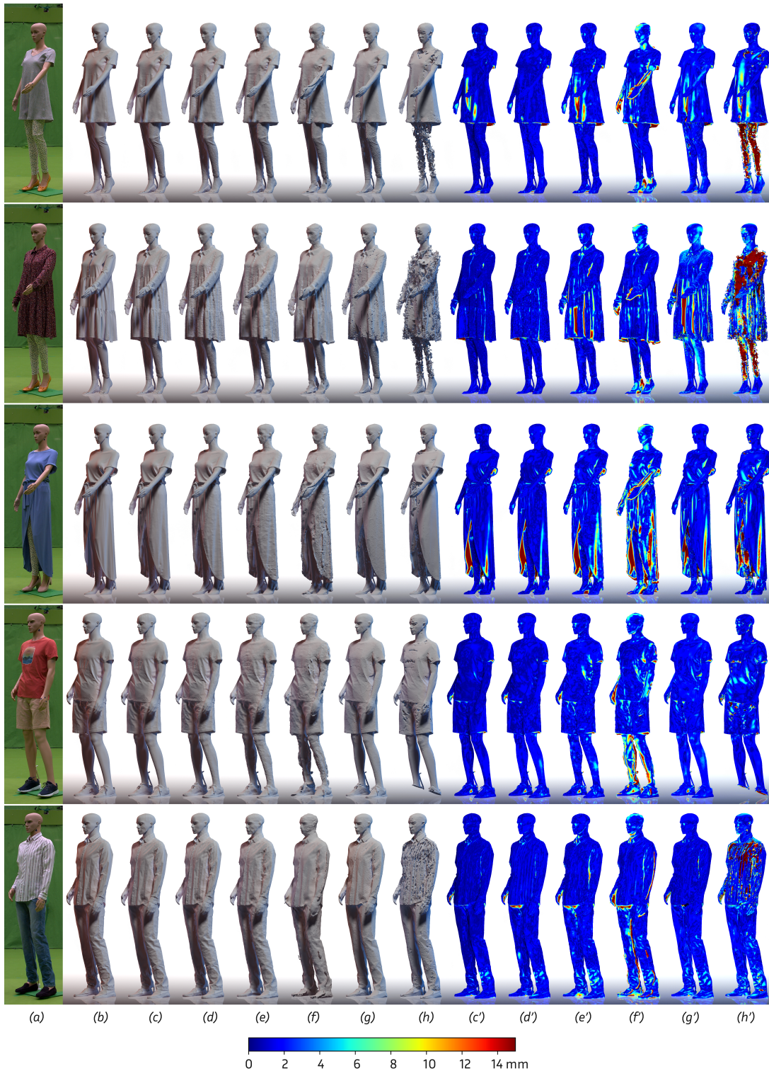
Fig. 8. Reconstructions on a subset of our proposed dataset with (a) input image, (b) reference scan, (c) our method, (d) Voxurf, (e) NeuS2, (f) Colmap, (g) 2DGS, (h) GOF and their associated accuracy heatmaps.
