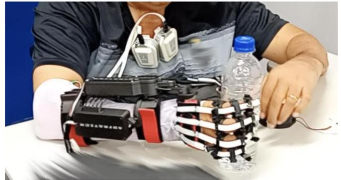
Figure 4: Position of the arm and object being held during the clinical test.
