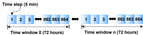
Fig. 2. Offline modules plan the actions for the next three days (time window).
