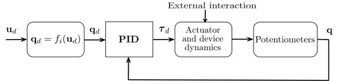
Figure 13: Position control system. The reference configuration is provided in the end-effector configuration space  $\mathbf{u}_d$ . The inverse kinematics procedure described in Sec. 3 allows to convert the desired configuration in the joint space. Finally, a PID controller is implemented, providing the desired motor torque  $\tau_d$ . The actual joint configuration is measured by the potentiometers placed on the device active joints ( $C, D, E, F$  – see Fig. 2).
