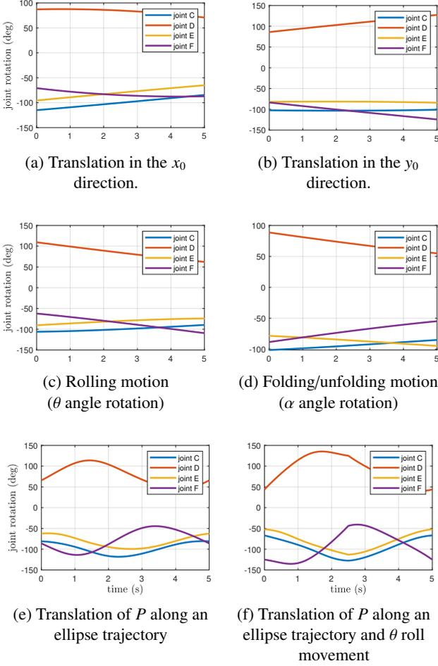
Figure 7: Numerical simulations: Rotation angles of actuated joints  $C, D, E, F$  as a function of time.
