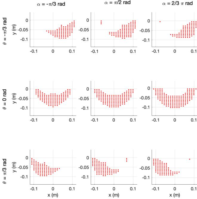
Figure 11: Numerical simulations: workspace evaluation. Dotted areas in the diagrams represent  $P$  point positions that can be reached for three different values of  $\theta$  ( $\theta = [-\pi/3, 0, \pi/3]$  rad, represented by rows) and  $\alpha$  ( $\theta = [\pi/3, \pi/2, 2/3\pi]$  rad, represented by columns).
