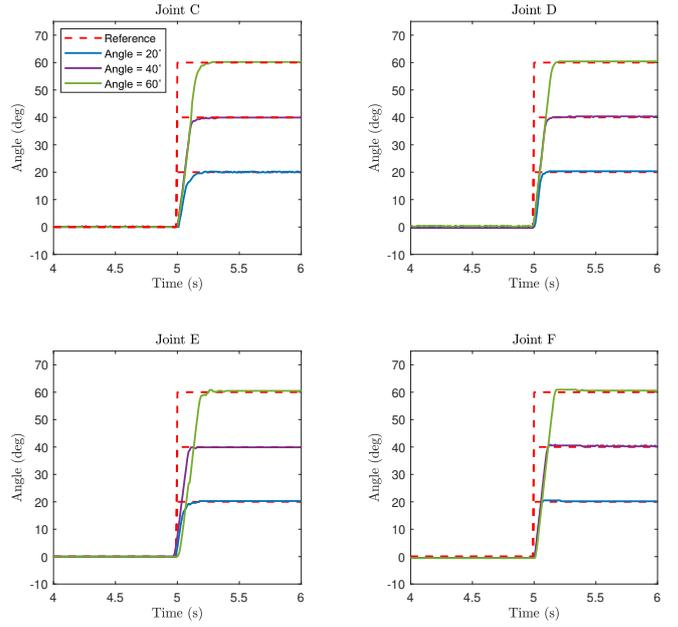
Figure 14: Step response. We commanded the four actuated joints to follow a step command, rotating from 0° to 20°, 40°, or 60°.
