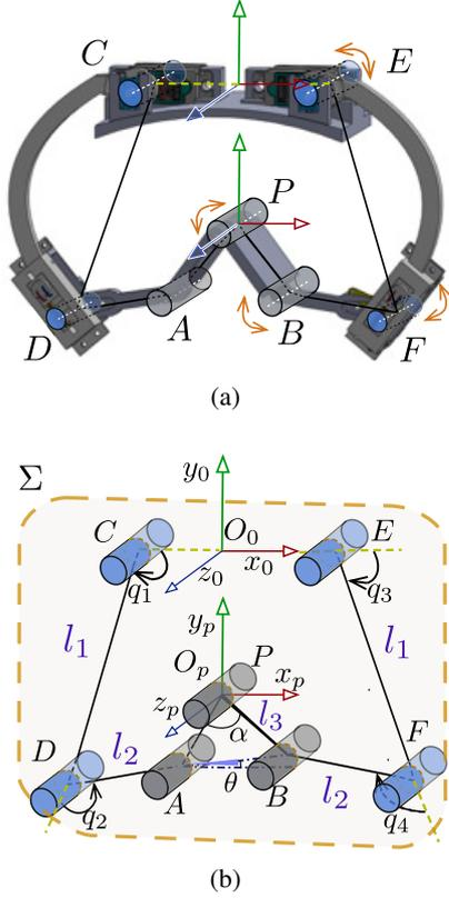
Figure 4: Kinematic structure of the proposed 4-DoF wearable haptic device. Two planar Revolute-Revolute chains, actuated by four motors, move the end-effector of the device. The position  $(x_p, y_p)$  of the middle point of the cylindrical bearing on the end-effector  $P$ , the roll angle  $\theta$  with respect to the  $x_0 - z_0$  plane, and the folding angle  $\alpha$  define the device active movements.
