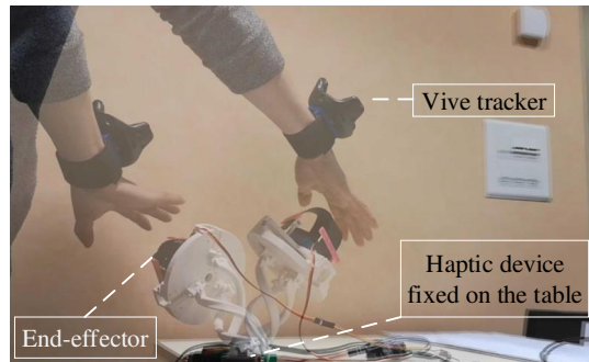
Fig. 11. Use case: encounter-type interaction with re-configurable surfaces. The motion of the user’s hand was tracked by the HTC Vive motion system. The base platform of the device was fixed on a table and the moving platform follows the hand so as to always face the user’s palm, ready for interaction.
