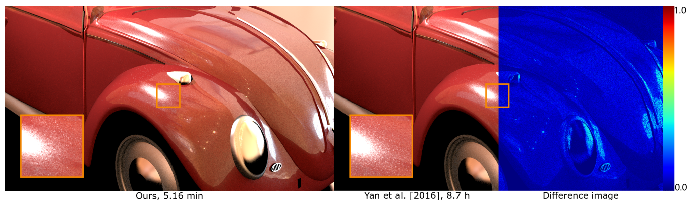
Fig. 1. Comparison between our method and Yan et al. [2016] on the Car scene, using a seamlessly tileable normal map of metallic flakes with resolution 2K \times 2K under geometric optics. The rendered glints are almost identical, but our method costs less than 1% of time compared to Yan et al. [2016], and does not scale with the view distance.
