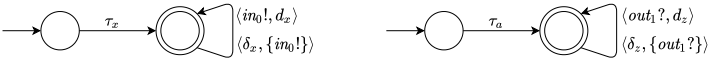
Fig. 8. FSMs of traces of \text{init}_{x_0} \circledast (\text{put}_x \sqcap \text{ode}_0)^* (left) and \text{init}_{a_0} \circledast (\text{get}_z \sqcap \text{ode}_1)^* (right)
