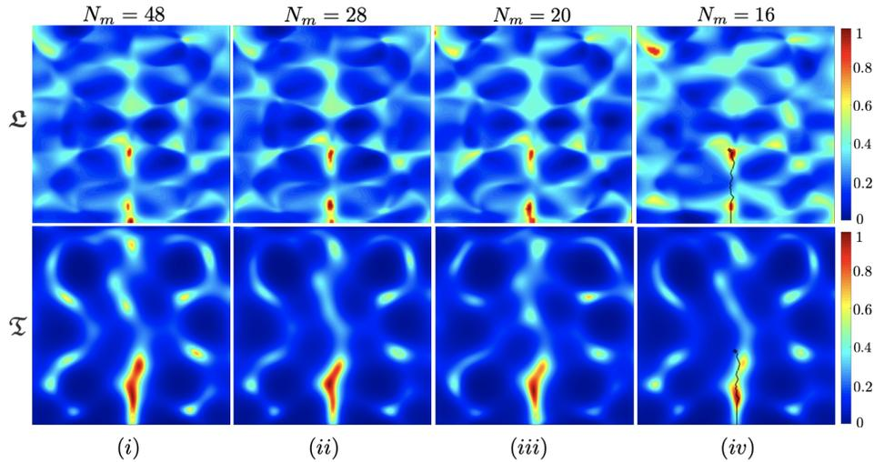
Figure 4: Time- vs. frequency- domain inversion from reduced data at 60% of the maximum load: (top) multifrequency indicator  $\mathfrak{L}$  [23], and (bottom) time-domain indicator  $\mathfrak{I}$ . Here, the number of scanning points on  $\Gamma_m$  is  $N_m$ .
