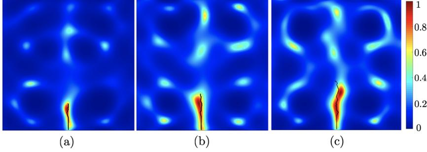
Figure 1: Time-domain reconstruction of an advancing fracture: (a-c)  $\mathfrak{T}$  maps computed from ultrasonic waveforms measured at 90%, 75%, and 60% of the maximum load in the post-peak regime. The solid line shows the ground truth.
