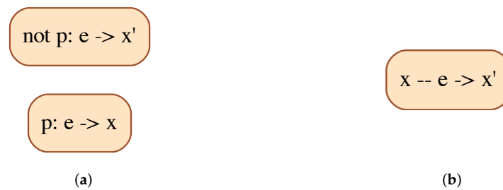
Figure 2. CDG and DG of the two-equation model from Figure 1. Vertices are conditional equation blocks of the form p: R - E \rightarrow W , where: E is the block of equations; p is a Boolean condition, defining the set of modes in which the block has to be solved; R is a set of variables to read, or free variables, i.e., parameters of the block of equations; W is a set of variables to write, meaning that they are the unknowns of the block of equations. When R is empty, the shorthand notation is p: E \rightarrow W . When p is the constant T , prefix “ p: ” is omitted. (a) CDG of the two-equation model, resulting from the multimode structural analysis; (b) DG of the two-equation model, resulting from the approximate structural analysis.
