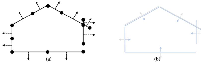
Figure 4: Disassembling of a CityGML model. Each facet of an input CityGML model (a) is duplicated and inverted. The class *outside* is assigned to each input facet while the class *inside* is assigned to the duplicated ones (b). Color code: input facets associated with the class *outside* in grey, duplicated ones associated with the class *inside* in blue.
