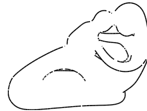
Fig. 4. Naive visibility. In this example, the occluding contour has been sampled into line segments, and then visibility for each segment was computed by a separate ray test against a dense triangulation of the surface. This naive strategy produces unreliable visibility, such as incorrect gaps in the contours. Most algorithms use a combination of heuristics that can greatly improve over a naive result, but they cannot remove all visibility errors. (Fertility by UU from AIM@SHAPE-VISIONAIR Shape Repository).
