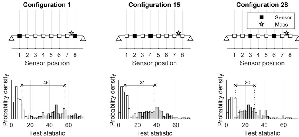
Figure 13: Optimizing the test sensor layout using  $T_8$  (based on simulated data) and comparing the test response for real data with  $\Delta_8 = 5\%$
