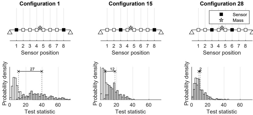
Figure 12: Optimizing the test sensor layout using  $T_5$  (based on simulated data) and comparing the test response for real data with  $\Delta_5 = 5\%$
