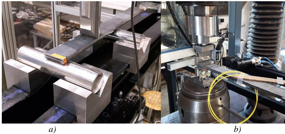
Figure 4. a) Photo of the ENF sample and test bed, b) Photo of the DCB sample and test bed.
