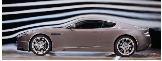
Fig. 24. Wind-tunnel test of a car. A wind tunnel visualization of the airflow around a car shows that the design of the body delays boundary layer separation until the trunk, which reduces drag and vibration in practice. Image courtesy of Auto Motor und Sport , ©Frank Herzog/Sportauto.
