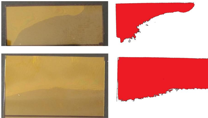
Fig. 11. Image processing applied to peeled samples. ROI (Region of Interest) original image (left) and processed image (right) for calculation of peeled area, in white. Runs reported: 100 A (a=10; e=0; sample A) on top and 150C (a=15; e=0, sample C) on bottom.
