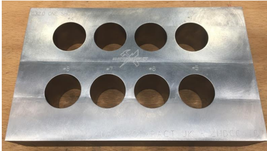
Fig. 5. 32.0mm Test Coupon A (Guehring Tipped Drill)
