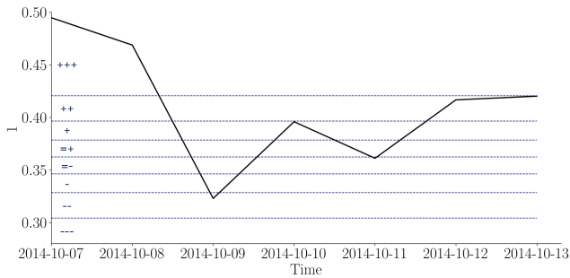
Figure 4: SAX discretization example on a rumination time series of length 7 with an alphabet of size 8.
