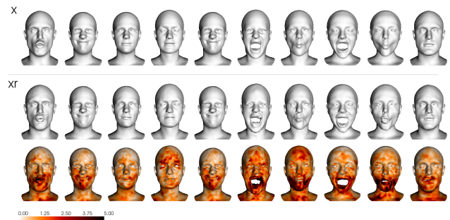
Figure 5: Reconstruction examples on CoMA. The first row shows the input mesh. The reconstruction is displayed in the second row, while the third row shows an error map relative to the input. Values are in millimeters.
