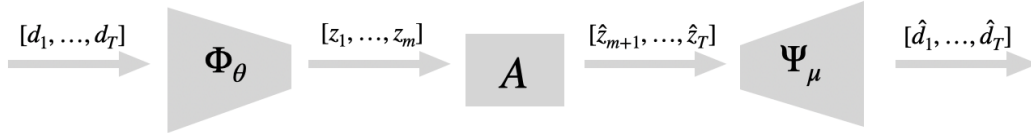
Figure 1: General overview of the proposed pipeline: the measurements [d_1, \dots, d_T] are first encoded with \Phi_\theta to codes [z_1, \dots, z_m] . Only the m first codes are used to estimate the linear system dynamics A arising from the least-squares minimization problem (3). Using this linear dynamics A and the last code z_m , the last T - m codes are predicted. The resulting reconstructed measurements [\hat{d}_1, \dots, \hat{d}_T] are obtained by decoding with \Psi_\theta the embeddings of the actual measurements [z_1, \dots, z_m] and the predicted embeddings [z_{m+1}, \dots, z_T] .
