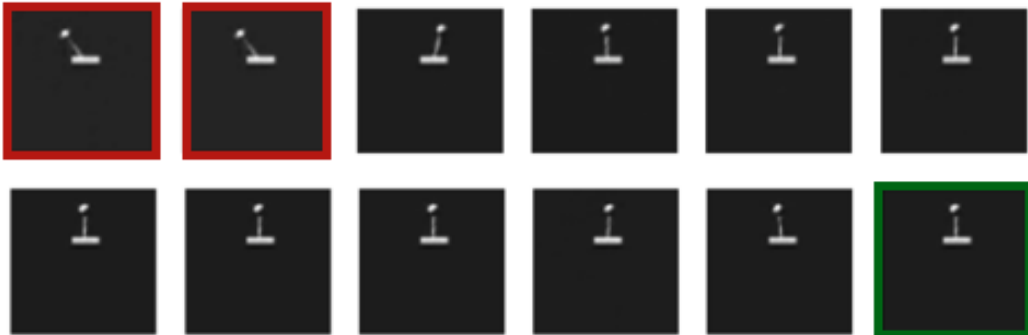
Figure 13: Illustration of cartpole control. Starting from an initial state specified by two consecutive frames (in red), we estimate and apply the controls necessary to guide the pole to an inverted position in a horizon of 0.5 s. The last frame shows the final position of the cartpole after all controls were applied (in green).
