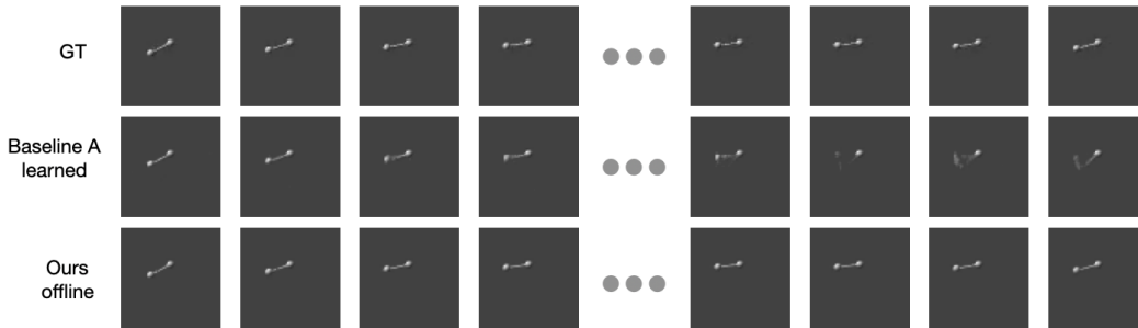
Figure 8: Prediction for the pendulum with low oscillations amplitude (between \frac{\pi}{2} and \frac{3\pi}{2} radians) and length 0.6 m. The first row shows ground truth (GT) images. The second row shows predicted frames without updates with the baseline model where the matrix A is a learned parameter. The third row is our model without updates.
