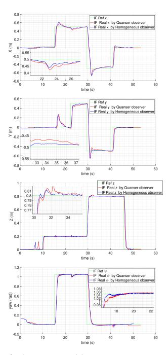
Figure 2: Quadrotor position stabilization comparisons in  $x,\,y,\,z$  and  $\psi$
