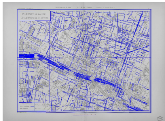
Fig. 5. Line segment extraction at high resolution: visual clues for graticule lines detection (6424 detected segments)
