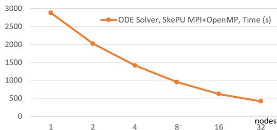
Fig. 12. Execution time (secs) of the SkePU 3 port of Variant A of the Embedded Runge-Kutta ODE solver implementation in the *Libsolve* library [33], solving the Brusselator 2D-MIX problem for system size  $3000 \times 3000$  on up to 32 nodes of *Tetralith*, using the MPI+OpenMP backend of SkePU.
