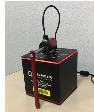
Fig. 2. Schematics and photo of the rotary inverted pendulum.
