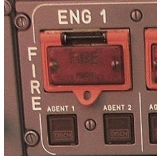
Fig. 4. Engine 1 FIRE push-button on the overhead panel.
