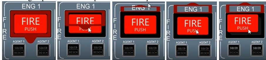
Fig. 5. Interactions sequence for pushing overhead panel-like FIRE push button
