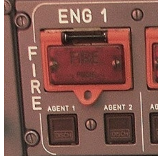
Fig. 4. Engine 1 FIRE push-button on the overhead panel.
