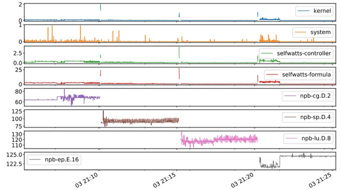
Fig. 3. Power estimations per VM for SEQUENTIAL phase
