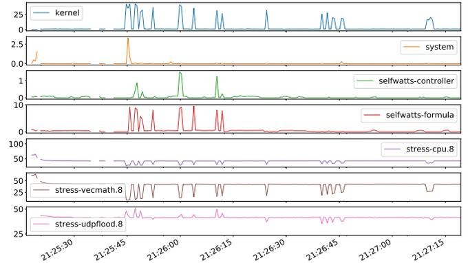
Fig. 4. Power estimations per VM for PARALLEL phase
