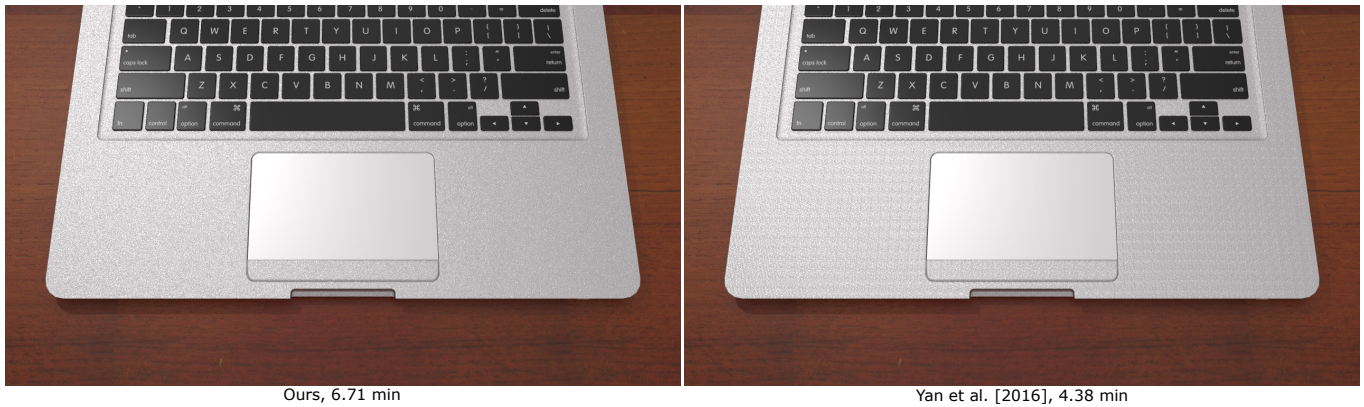
Fig. 9. Comparison between our method and Yan et al. [2016] with a tiled texture on the Laptop Scene. The repeated pattern is visible in Yan et al. [2016]. Normal map: isotropic noise.
