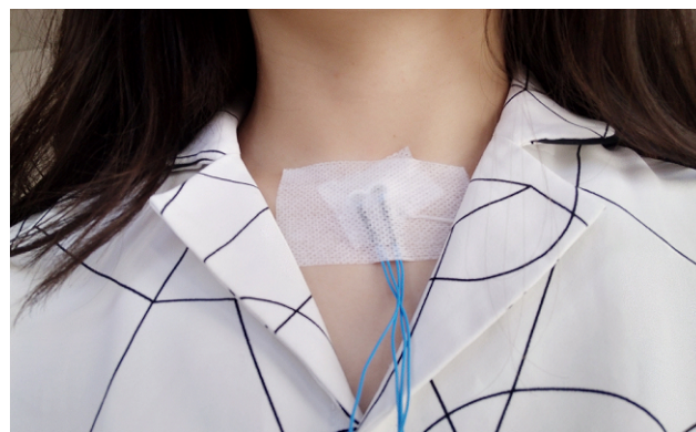
Figure 2. Position of the microphones: two microphones are inserted into the support that is fixed at suprasternal notch with two strips of adhesive tape.
