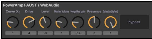
Figure 14: GUI generated by the FAUST IDE, some extra parameters (negative feedback gain, waveshaper; drive, curve, saturation) are tweakable, enabling fine tuning of the NFB loop.
