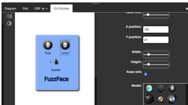
Figure 5: a default GUI is proposed from a FAUST code in the editor.
