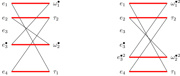
Figure 15: The clutch is an example in which c_f^- = c_f holds. Maximal cardinality matchings for N = 1 (left) and N = 2 (right) are given. Subsequently applying the Dulmage-Mendelsohn decomposition returns \beta_{\mathcal{D}} = \{e_3\} on the left, and \beta_{\mathcal{D}} = \{e_3, e_3^{\bullet}\} on the right.
