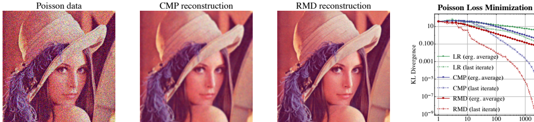
Figure 1: Reconstruction of the Lena test image from a sample contaminated with Poisson noise. Left to right: (a) the contaminated sample; (b) CMP reconstruction; (c) RMD reconstruction; and (d) Poisson likelihood loss at each iteration. The RMD process provides a sharper definition of image features relative to the CMP algorithm (which is the second-best); higher-definition images and more details can be found in the appendix.
