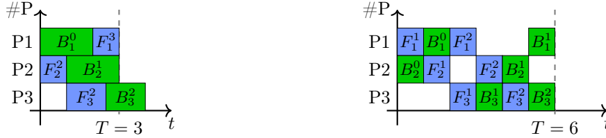
(a) 1-periodic pattern for the schedule of Figure 2. (b) 2-periodic pattern for 3 layers where u_F = u_B = 1 .
