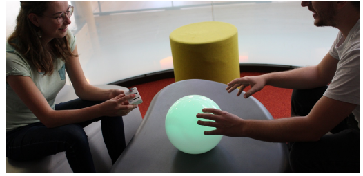
Figure 10: A person uses a brick stack to explore their heart activity via vibration (left) while also streaming the information to a light via Bluetooth (right orb).
