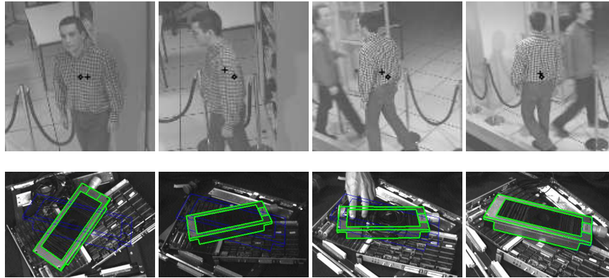
Fig. 1 Few images acquired during two visual servoing tasks: on the top, pedestrian tracking using a pan-tilt camera; on the bottom, controlling the 6 degrees of freedom of an eye-in-hand system so that an object appears at a particular position in the image (shown in blue).
