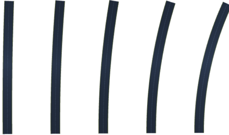
Fig. 2: Five different rotation gains applied to the travel path in our experiment. From left to right: \beta = 0.25, 0.5, 1, 1.75, and 2.5 degrees, respectively.
