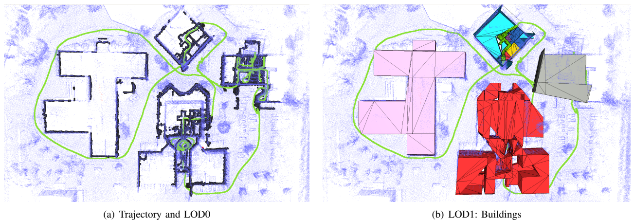
Fig. 7. Indoor 3D reconstruction and indoor/outdoor localization example. Two LOD are provided along the estimated trajectory (in green) and the aligned pointcloud (in blue): a) Floorplan for the first stage of each building is shown in black. b) Extrusion of detected buildings by using the algorithm [20] For the building in blue, the indoor information is the LOD1 presented in Fig. 6.
