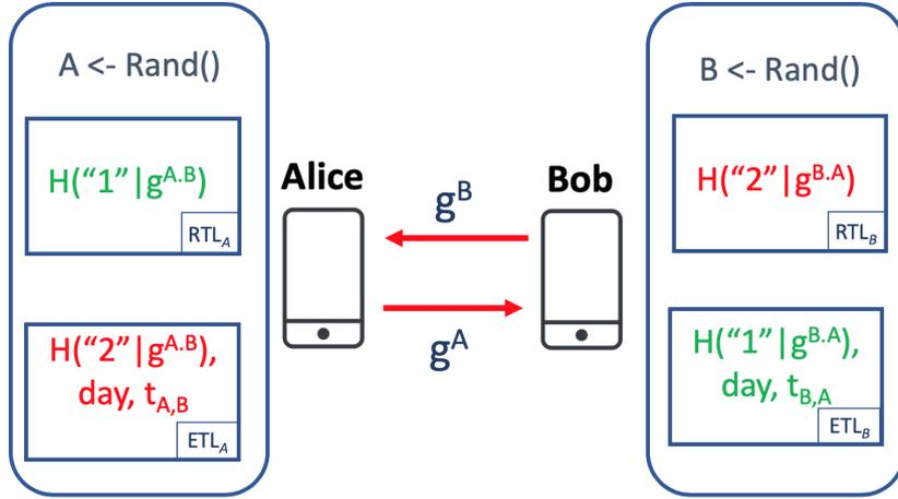
Figure 2: Device  $A$  broadcasts  $EBID = g^A$ . Device  $B$  broadcasts  $EBID = g^B$ . Device  $A$  computes  $PET^1 = H("1" | g^{B,A})$  and  $PET^2 = H("2" | g^{B,A})$ , stores  $PET^1$  in  $RTL_A$  and  $PET^2$  in  $ETL_A$ . Device  $B$  computes  $PET^1 = H("1" | g^{A,B})$  and  $PET^2 = H("2" | g^{A,B})$ , stores  $PET^1$  in  $ETL_B$  and  $PET^2$  in  $RTL_B$ .
