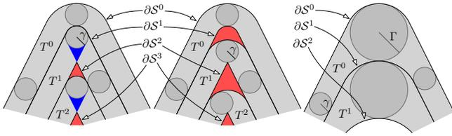
Fig. 2. *Left.* Uniform-width contouring. Beads have constant width  $2\gamma$  and produce overfill as self-overlap in the blue areas. The inner red areas are not covered: we have underfill. *Middle.* Regularized parallel contouring avoids overfill. Beads have constant width  $2\gamma$ . *Right.* Variable-width contouring (our technique) models beads with varying width in the range  $[2\gamma, 2\Gamma]$ .
