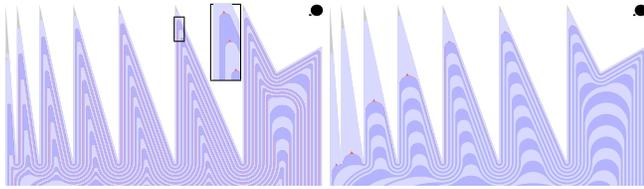
Fig. 12. Illustrating the collapse heuristics. The input shape shows 8 spikes ordered from left to right. *Left*. Base collapse only, up to  $4\gamma$ , with  $2\gamma = 0.08$  and  $2\Gamma = 0.5$ . *Right*. The full collapse heuristics.
