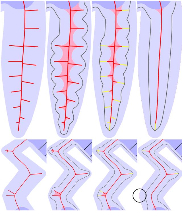
Fig. 10. Two parts of the funny figure of Figure 17. *From left to right:* The labeled MA ( $S^0$ ); Gaps without shaving nor medial axis simplification; With shaving (the yellow color indicates *Shaved* arcs); With both. The circle highlights gaps due to a local loss of shape fidelity.
