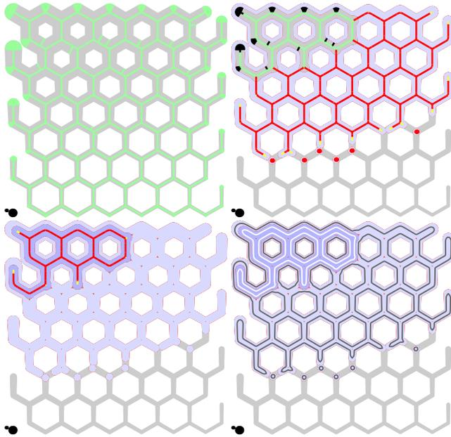
Fig. 15. A complex collapsed axis. In reading order: The input polygon and its medial axis. The labeled medial axis  $MA(S^0)$ . The labeled medial axis  $MA(S^1)$ . The resulting two beads and their trajectories (black for  $T^0$ , white for  $T^1$ ).
