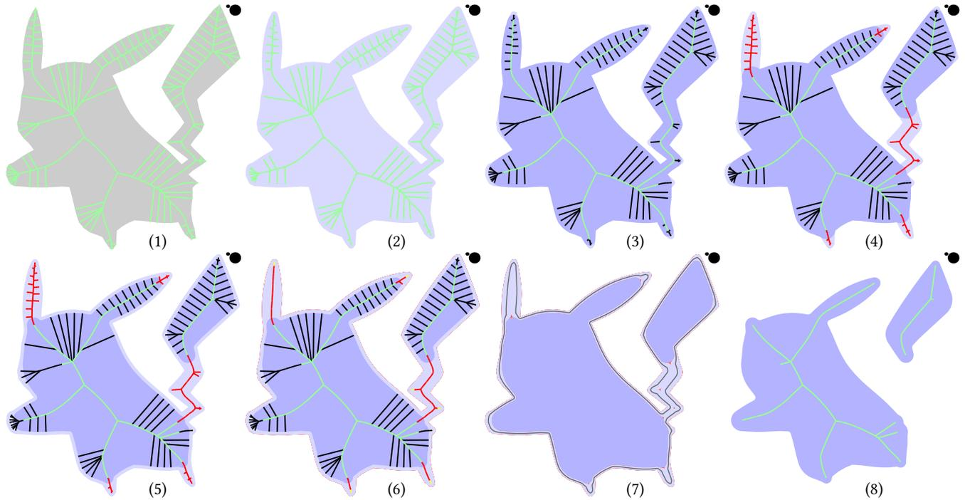
Fig. 17. The bead width range is  $[0.3, 1.0]$ . The dark blue shape is generated by  $Normal(MA(S^0))$ . In reading order. 1: The input polygon and its medial axis. 2: Shape  $S^0$  and its medial axis. 3: Trimming. 4: Collapsing. 5: Parallel offset (only  $d_{S^0}$  is modified: the dark blue shape is  $S^1$ ). 6: Medial axis simplification and shaving. 7: Sampling of  $\text{traj}(T^0)$ . 8: The medial axis of  $S^1$  is much simpler.
