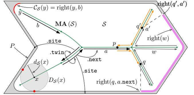
Fig. 5. Some notation. The wide black arrows along the medial axis are half-arcs. The bottom-left red dots are the contact points  $C_S(x)$  of  $x$ . The gray half-arcs form the walk  $w$  from point  $q$  on  $a$ .next to point  $q'$  on  $a'$ . The right-curve of  $w$ ,  $\text{right}(w)$ , is drawn in violet. Together, the gray and orange half-arcs form the  $w$ -tree  $\mathcal{T}_{p,a}$  (defined in Section 5).
