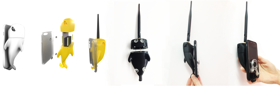
Fig. 1. Seamote Bridge. An evolution of special design case with the embedded microcontroller and LoRa antenna, capable to be mounted to the smartphone using suction cups.
